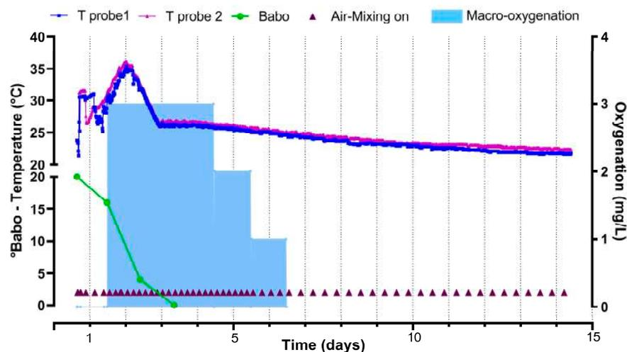
**Figure 3.** Evolution of tank temperature (°C) and sugar content (°Babo) during the winemaking process managed by the Air-Mixing system and macro-oxygenation (the triangles indicate when Air-Mixing turns on).
